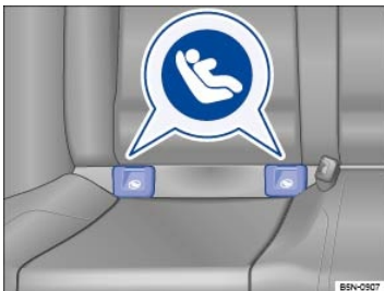
Fig. 43 On the second row outboard seat backrests: Markings indicating the location of the LATCH/UCRA lower universal anchorages.
