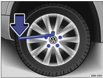
Fig. 197 Changing a wheel: Loosening the wheel bolts.
