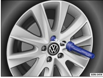
Fig. 201 Changing a wheel: Remove previously loosened wheel bolts using the screwdriver handle.
