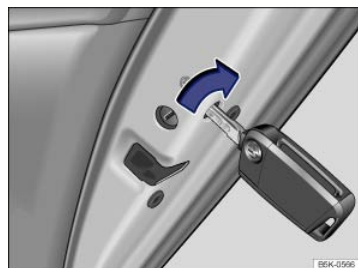
Fig. 59 On the front side of the rear passenger door: Locking the vehicle with the key bit in the vehicle key.
