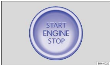
Fig. 112 In the lower center console: Starter button for the Keyless Access system.
