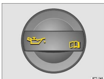
Fig. 185 In the engine compartment: Engine oil filler cap (cap design may vary depending on vehicle equipment).
