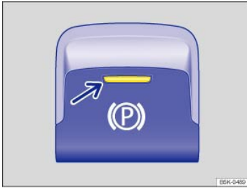
Fig. 134 In the lower center console: Electronic parking brake switch.
