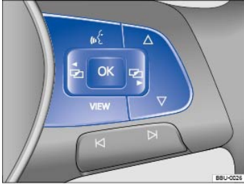
Fig. 17 Right side of the multi-function steering wheel: Controls for the menus and information in the instrument cluster display.
