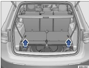
Fig. 153 In the luggage compartment for vehicles with seven seats: Pull straps to lift third row bench and access the subwoofer.
