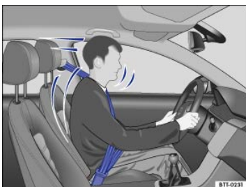
Fig. 25 Belted driver secured by the correctly worn safety belt in the event of a sudden braking maneuver.
