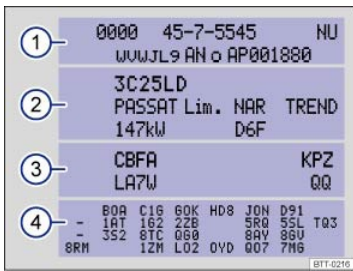
Fig. 204 Vehicle identification label: Shown in the example with engine identification code CBFA ③.
