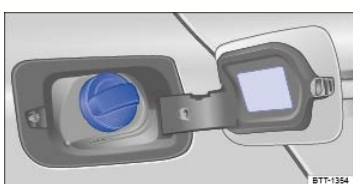
Fig. 166 Rear passenger side of vehicle: Fuel cap placed on the open fuel filler flap.
