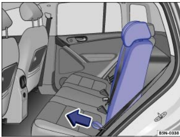
Fig. 78 In the second row: Pull strap to fold the second row backrest forward.
