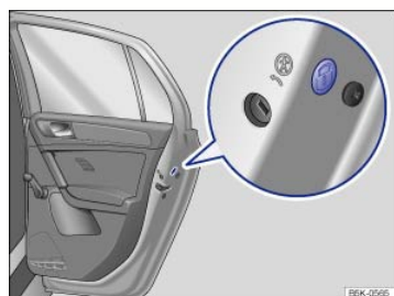
Fig. 58 On the front side of the rear passenger door: Manual lock, covered by a rubber seal.
