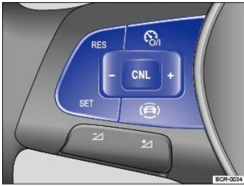
Fig. 126 Left-hand side of the multi-function steering wheel: Buttons for operating the cruise control.
