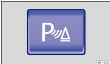
Fig. 135 In the lower center console: Button to switch the Park Distance Control system on or off (vehicles without Area View).
