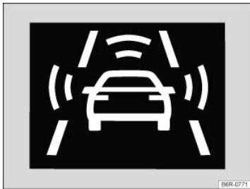
Fig. 131 In the instrument cluster display: Advance warning (symbol displayed in color on an instrument cluster with color display).
