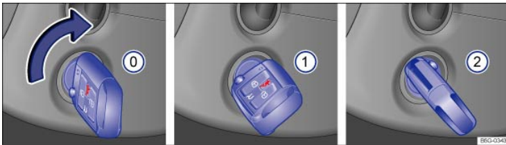
Fig. 111 In the ignition switch: Vehicle key positions for vehicles without Keyless Access.
