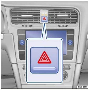
Fig. 46 In the center of the instrument panel: Button for the emergency flashers.
