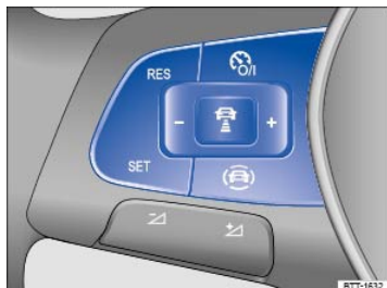
Fig. 129 Left-hand side of the multi-function steering wheel: Buttons for operating the Adaptive Cruise Control (ACC).
