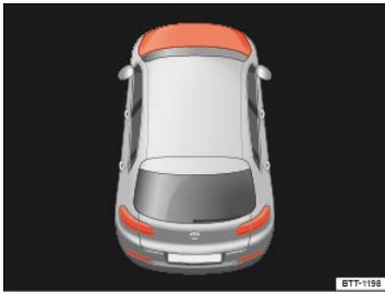
Fig. 182 In the instrument cluster display: Engine hood open or not properly closed.
