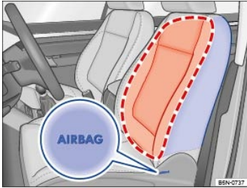
Fig. 35 Location and deployment zone of the side airbags in the padding on the outboard side of the front seat backrests.
