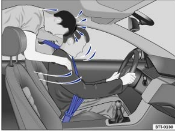
Fig. 24 Unbelted passengers in the rear seats are thrown forward on top of the belted driver.
