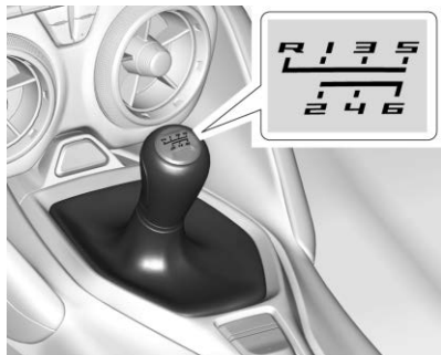
Shift Pattern – I4 and V6 Engines
