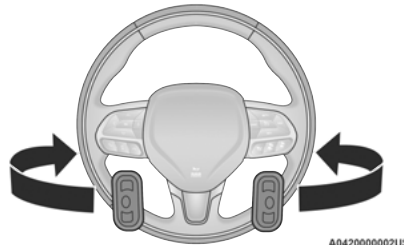
Remote Sound System Controls
