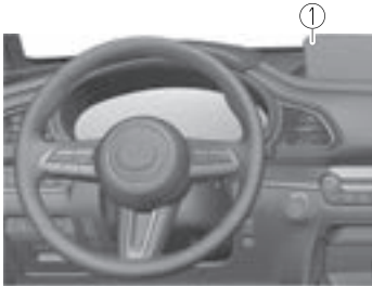
1. Driver monitoring camera
