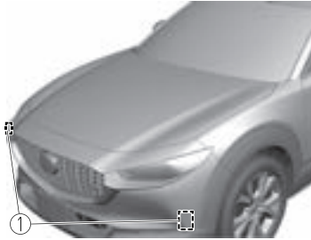
1. Front side radar sensor
