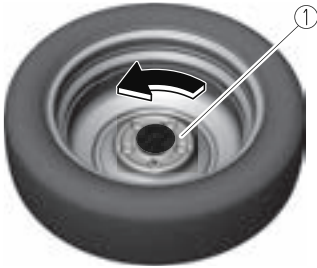
1. Spare tire hold-down bolt
