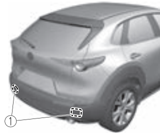
1. Rear side radar sensor
