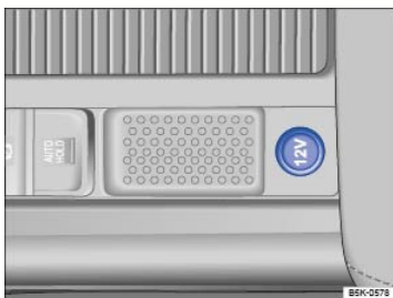
Fig. 133 In the lower center console: 12 Volt socket (vehicles with electronic parking brake).
