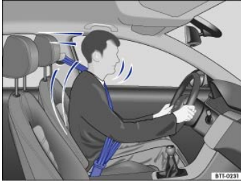
Fig. 61 Belted driver secured by the correctly worn safety belt in the event of a sudden braking maneuver.
