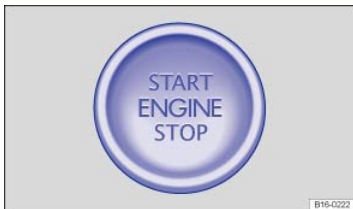
Fig. 135 In the lower center console: Starter button for the Keyless Access system.
