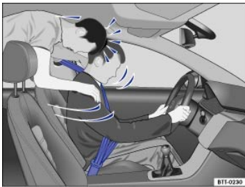
Fig. 60 Unbelted passengers in the rear seats are thrown forward on top of the belted driver.
