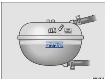
Fig. 201 Coolant expansion tank in the engine compartment.
