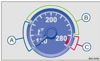
Fig. 200 Engine coolant temperature gauge in the instrument cluster: Ⓐ Engine cold; Ⓑ Normal temperature range; Ⓒ Warning zone.
