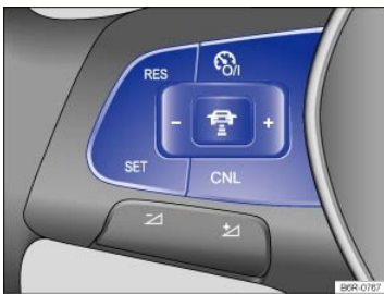
Fig. 160 Left-hand side of the multifunction steering wheel: Buttons for operating the Adaptive Cruise Control (ACC).
