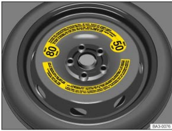
Fig. 115 In the luggage compartment: Compact spare wheel (if equipped, label design may vary).
