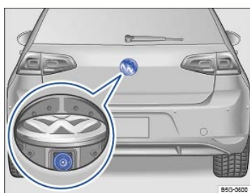
Fig. 169 In the trunk lid: Location of the camera.
