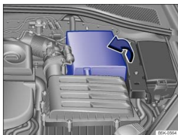
Fig. 203 In the engine compartment: Open the sleeve covering of the vehicle battery.
