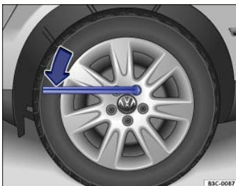
Fig. 222 Changing a wheel: Loosening the wheel bolts.
