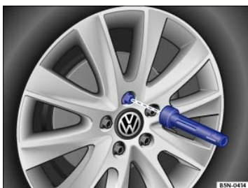
Fig. 229 Changing a wheel: Remove previously loosened wheel bolts using the screwdriver handle.
