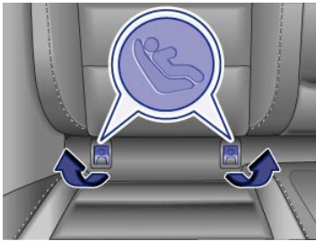
Fig. 80 On the rear outboard seat backrests: Markings on the covers of the LATCH/UCRA lower universal anchorages.
