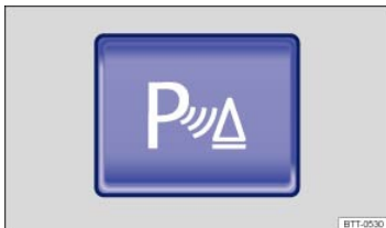
Fig. 173 In the lower center console: Button to switch the Park Distance Control system on or off.
