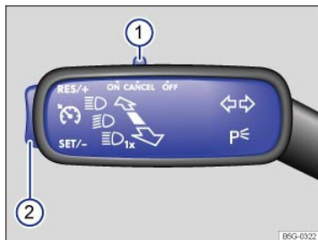
Fig. 154 On the turn signal lever: Cruise control buttons and switches (if equipped).
