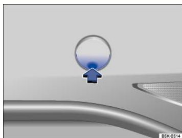
Fig. 239 In the right rear bumper: Removing the cover.
