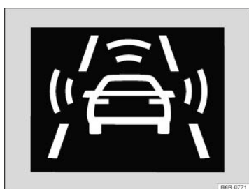
Fig. 164 In the instrument cluster display: Advance warning (symbol displayed in color on an instrument cluster with color display).
