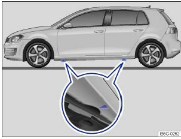
Fig. 226 Lift points for the jack.
