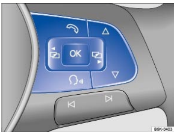
Fig. 17 Right side of the multi-function steering wheel (if equipped): Controls for the menus and information in the instrument cluster display.
