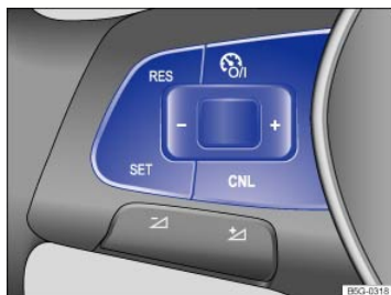
Fig. 155 Left-hand side of the multi-function steering wheel (if equipped): Buttons for operating the cruise control.
