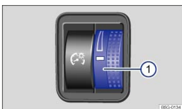
Fig. 87 To the left of the steering wheel: Thumbwheel to adjust instrument panel lighting ①.
