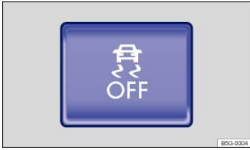
Fig. 147 In the center console: Button for switching ASR or ESC Sport mode on and off manually (if equipped).
