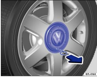
Fig. 218 Pulling the hubcap off.
