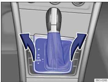
Fig. 214 Removing the selector gate cover.
