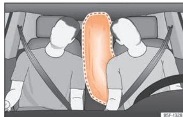
Fig. 25 Fully inflated central airbag (deployment zone).
