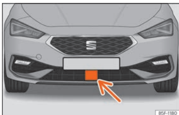
Fig. 171 On the front bumper: radar sensors.
