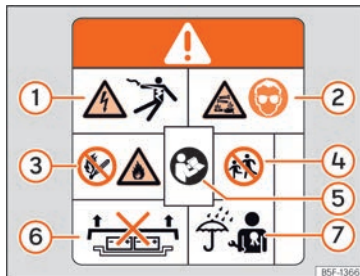
Fig. 212 High-voltage battery warning lettering.
