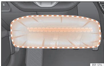
Fig. 23 On the driver side: airbag action radius for the knees.
