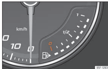
Fig. 68 Analogue instrument panel: fuel gauge
