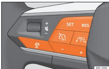
Fig. 190 Left side of the multifunction steering wheel: buttons for operating Travel Assist.
