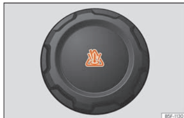
Fig. 236 Engine compartment: coolant expansion tank cap.
