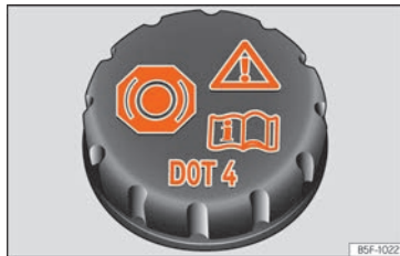
Fig. 237 Engine compartment: brake fluid reservoir cap.
