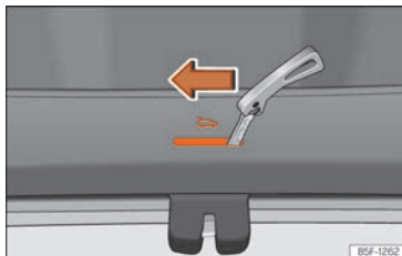
Fig. 98 Detail of the luggage compartment: emergency release (Leon).
