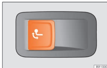
Fig. 209 On the left side of the luggage compartment: button for unlocking the tow hook.
