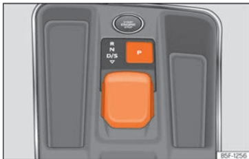
Fig. 169 In the centre console: selector lever.
