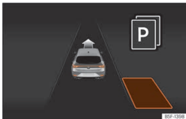
Fig. 200 On the instrument panel display: view of the parking assist system with reduced view.
