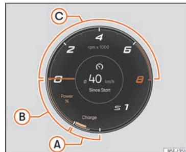
Fig. 66 Digital instrument panel: Power meter
