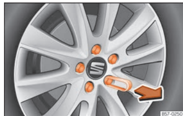
Fig. 42 Wheel: wheel nuts with caps.
