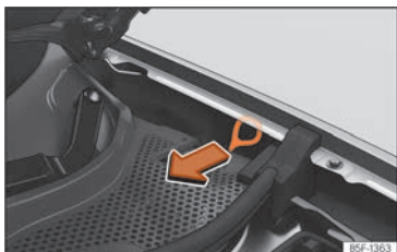
Fig. 218 Between the left wing panel and the engine bonnet hinge: Charging connector manual release mechanism puller.
