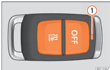
Fig. 155 Auxiliary heating: radio-operated remote control.
