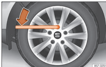
Fig. 44 Wheel change: loosen the wheel nuts.
