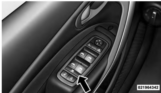
Window Lockout Switch
