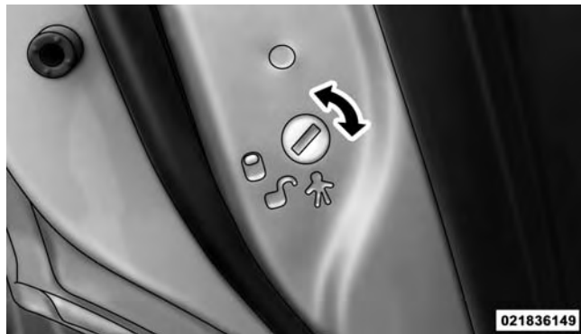
Child-Protection Door Lock Function
