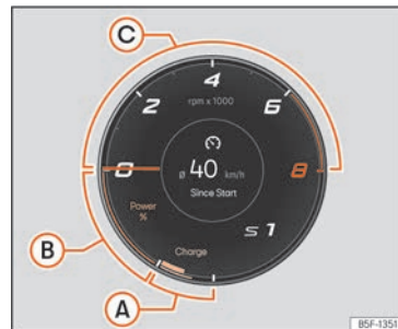
Fig. 65 Digital instrument panel: Power meter
