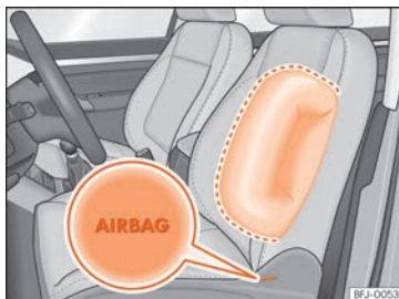
Fig. 26 Side airbag in driver's seat.
