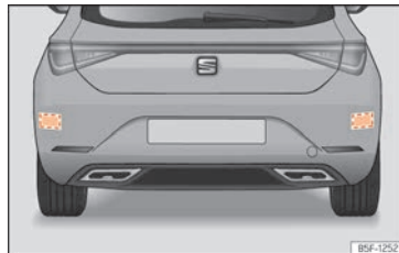
Fig. 172 Rear view of the vehicle: radar sensor zones.
