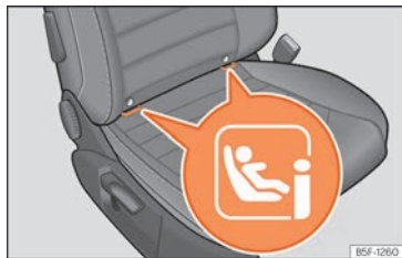
Fig. 33 Front passenger seat: ISOFIX/i-Size securing rings.
