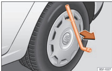
Fig. 40 Remove the wheel cover.
