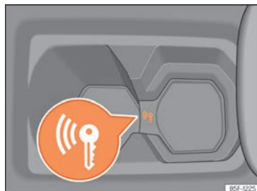
Fig. 164 In the centre console: emergency start.
