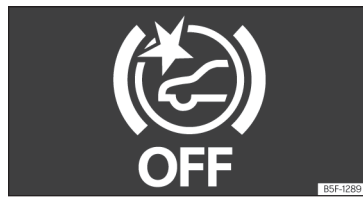
Fig. 179 On the instrument panel display: Front Assist deactivated indication.
