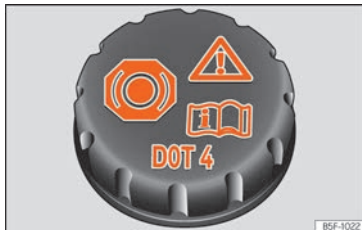
Fig. 235 Engine compartment: brake fluid reservoir cap.
