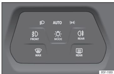
Fig. 102 Dash panel: lights control.
