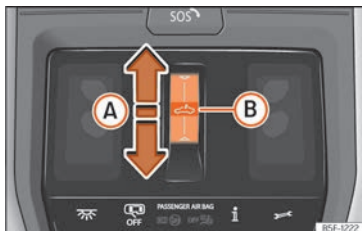
Fig. 100 On the interior roof lining: sunroof button.
