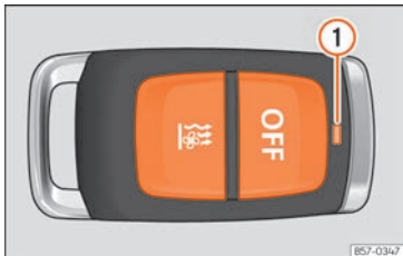
Fig. 153 Auxiliary heating: radio-operated remote control.
