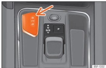
Fig. 82 Centre console: vehicle key socket.
