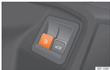
Fig. 220 Driver's door: tank flap release.
