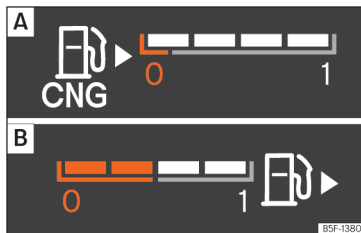
Fig. 69 Digital instrument panel: A : Natural gas gauge. B : Petrol gauge
