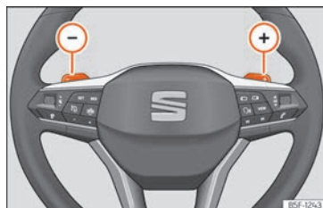
Fig. 168 Steering wheel: automatic transmission levers
