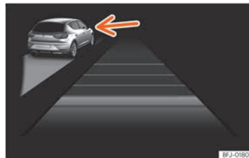
Fig. 182 On the instrument panel display: ACC active, vehicle detected in an outer lane.
