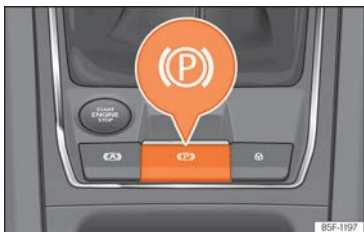
Fig. 196 In the lower part of the centre console: electronic parking brake button
