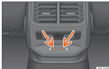
Fig. 162 Rear part of the centre console: USB connectors with power outlet function.
