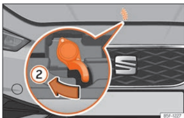
Fig. 226 Lever under the bonnet.
