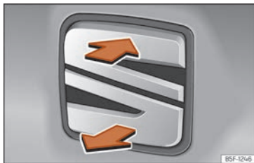
Fig. 93 Rear lid: opening from outside.
