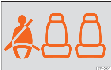
Fig. 10 Instrument panel: left rear seat occupied and corresponding seat belt fastened display.
