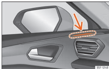
Fig. 189 Control lamp of the lane departure warning.
