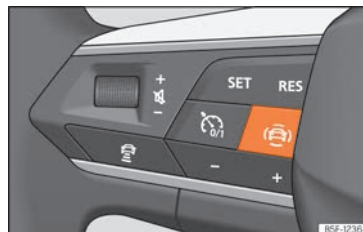
Fig. 73 Left side of the multifunction steering wheel: button for driver assistance systems (depending on versions).
