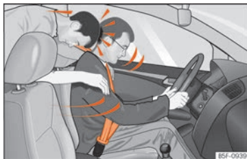
Fig. 13 The unbelted passenger in the rear seat is thrown forward violently, hitting the driver who is wearing a seat belt.
