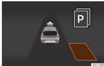
Fig. 198 On the instrument panel display: view of the parking assist system with reduced view.
