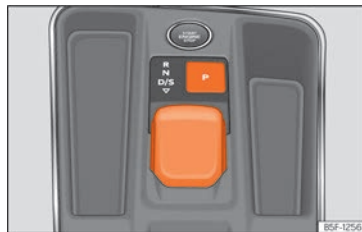
Fig. 167 In the centre console: selector lever.
