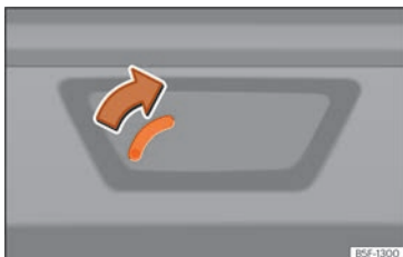
Fig. 98 Detail of the luggage compartment: manual release mechanism (Leon Sportstourer).
