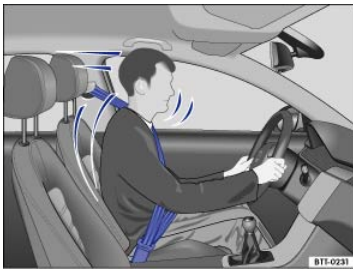
Fig. 55 Belted driver secured by the correctly worn safety belt in the event of a sudden braking maneuver.
