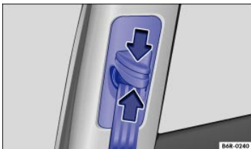
Fig. 60 Next to the front seats: Safety belt height adjuster.
