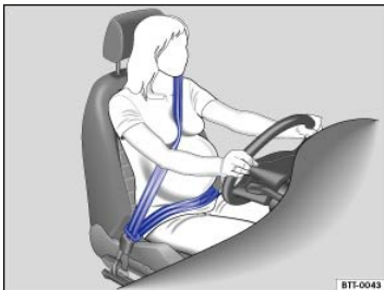
Fig. 59 Proper safety belt positioning for expectant mothers.
