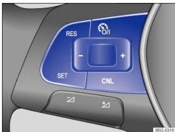
Fig. 124 Left-hand side of the multi-function steering wheel: Buttons for using the cruise control.
