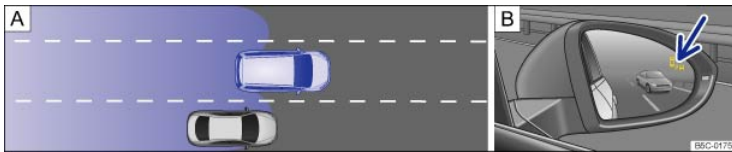
Fig. 150 : Driving situation when passing and merging into the lane. : Blind Spot Monitor indicator light in the passenger side mirror.
