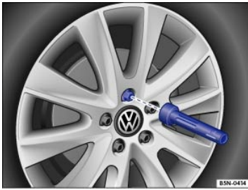
Fig. 183 Changing a wheel: remove previously loosened wheel bolts using the screwdriver handle.
