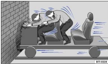
Fig. 52 A vehicle with passengers not wearing safety belts hits a wall.
