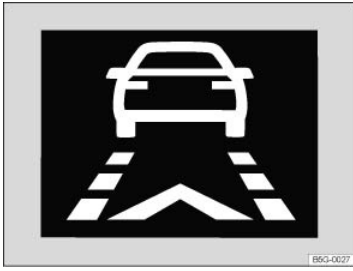
Fig. 133 In the instrument cluster display: Advance warning (symbol displayed in color on an instrument cluster with color display).
