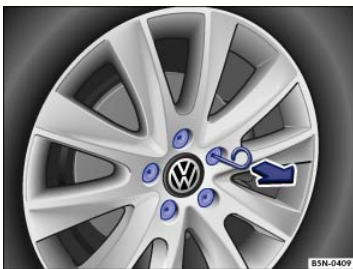
Fig. 177 Pulling cover caps off wheel bolts.
