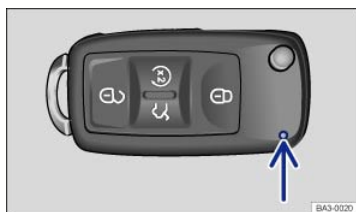
Fig. 16 Indicator light in the remote control vehicle key (version 2).
