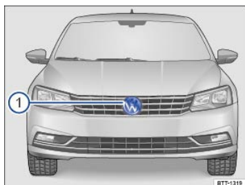
Fig. 134 In the front bumper: Radar sensor.
