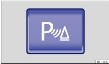
Fig. 142 In the lower center console: Button to switch the Park Distance Control system on or off.
