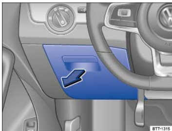
Fig. 184 On the driver side in the instrument panel: Fuse box behind the storage compartment.
