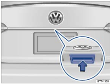
Fig. 27 Opening trunk lid from the outside.
