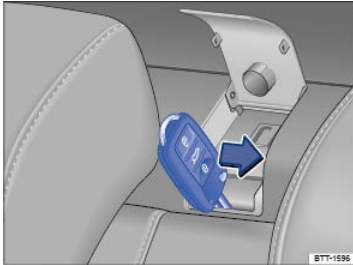
Fig. 30 Behind the rear seat backrest on the driver side: releasing the rear seat backrest.
