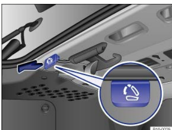
Fig. 90 On the left side of the luggage compartment: Release lever for the left-side rear seat backrest. The release lever for the right-side rear seat backrest is on the right side of the luggage compartment.
