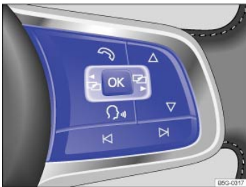
Fig. 11 Premium version (vehicles with menu control multi-function steering wheel): Buttons on the right side of the steering wheel.
