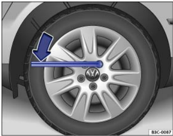
Fig. 179 Changing a wheel: Loosening wheel bolts.
