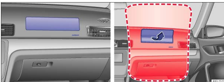
Fig. 65 Location and deployment zone of the front passenger front airbag.
