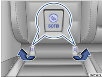
Fig. 73 On the rear outboard seat backrests: Removing the covers (if equipped) on the LATCH/UCRA lower universal anchorages.
