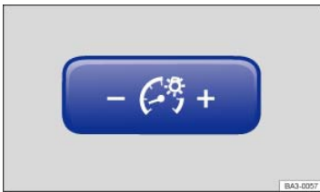
Fig. 79 To the left of the steering wheel: Control for instrument panel lighting.
