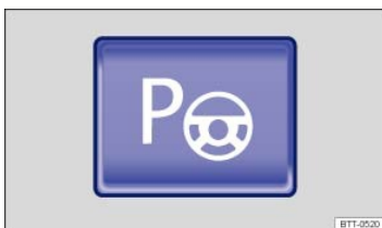
Fig. 144 In the lower center console: Button for switching on the Park Assist system.
