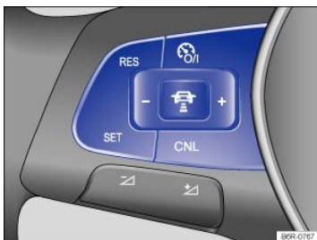
Fig. 129 Left-hand side of the multi-function steering wheel: Buttons for using ACC.
