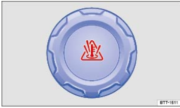
Fig. 163 Coolant expansion tank cap in the engine compartment.
