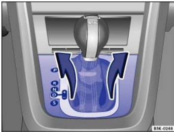
Fig. 175 Removing the selector gate cover.
