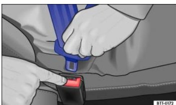
Fig. 57 Releasing the buckle tongue from the belt buckle.
