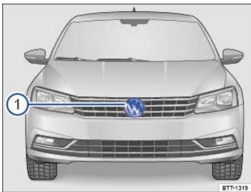
Fig. 127 Behind the Volkswagen emblem: Radar sensor.
