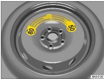
Fig. 99 In the luggage compartment: Compact spare wheel.
