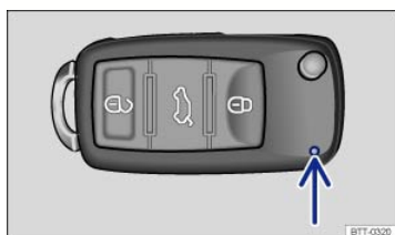
Fig. 15 Indicator light in the remote control vehicle key (version 1).
