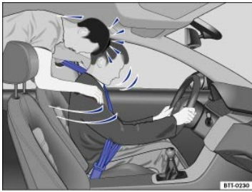
Fig. 54 Unbelted passengers in the rear seats are thrown forward on top of the belted driver.
