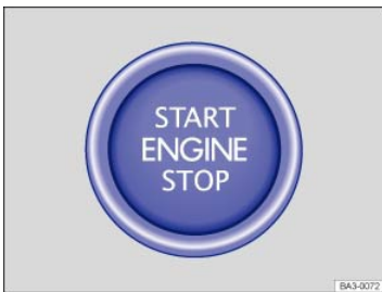
Fig. 112 In the center console: Starter button of the Keyless Access with push button start.
