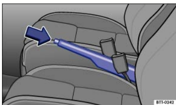
Fig. 119 Between the front seats: Parking brake.
