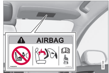
Alternative 1: Position of airbag label on passenger side sun visor.
