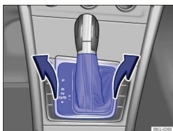
Fig. 107 Removing the selector gate cover.
