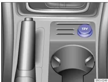
Fig. 143 In the lower center console: 12 Volt socket (vehicles with parking brake lever).
