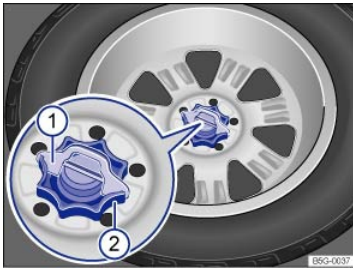
Fig. 184 In the luggage compartment: Handwheel holding the spare wheel in place (if equipped).
