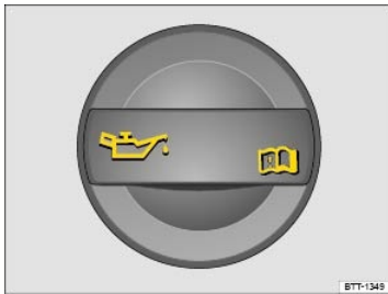
Fig. 177 In the engine compartment: Engine oil filler cap (cap design may vary depending on vehicle equipment).
