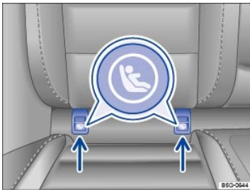
Fig. 47 On the rear outboard seat backrests: Markings on the LATCH/UAS lower universal anchorages.
