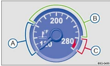
Fig. 15 Engine coolant temperature gauge in the instrument cluster.
