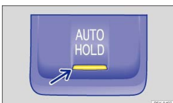
Fig. 120 In the lower center console: Button for Auto Hold (if equipped).
