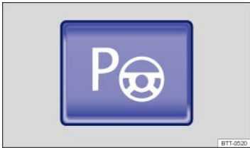
Fig. 124 In the lower center console: Button for switching on the Park Assist system.
