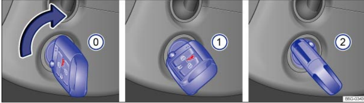
Fig. 99 In the ignition switch: Vehicle key positions for vehicles without Keyless Access.
