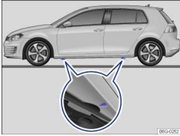
Fig. 195 Lift points for the jack.
