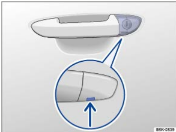
Fig. 56 Driver door: Concealed lock cylinder.
