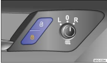
Fig. 55 In the driver and front passenger doors: Power locking switch.
