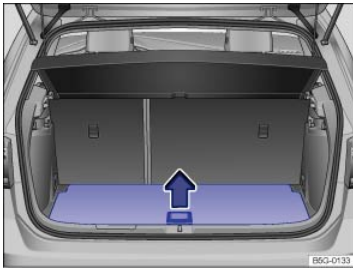
Fig. 148 In the luggage compartment: Opening the variable luggage compartment floor.
