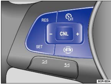
Fig. 110 Left-hand side of the multi-function steering wheel: Buttons for operating the cruise control.
