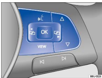
Fig. 19 Right side of the multi-function steering wheel: Controls for the menus and information in the instrument cluster display.
