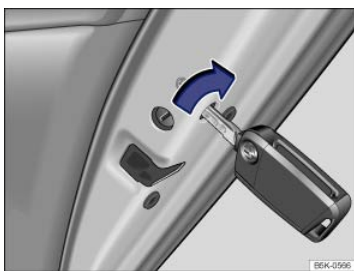
Fig. 59 On the front side of the rear passenger door: Locking the vehicle with the key bit in the vehicle key.
