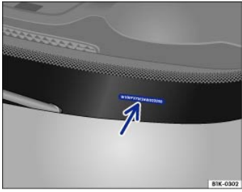
Fig. 202 Vehicle identification number (VIN).
