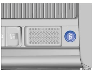
Fig. 144 In the lower center console: 12 Volt socket (vehicles with electronic parking brake).
