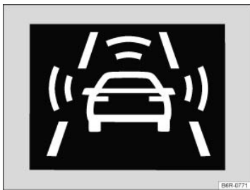
Fig. 115 In the instrument cluster display: Advance warning (symbol displayed in color on an instrument cluster with color display).
