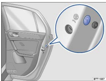
Fig. 58 On the front side of the rear passenger door: Manual lock, covered by a rubber seal.
