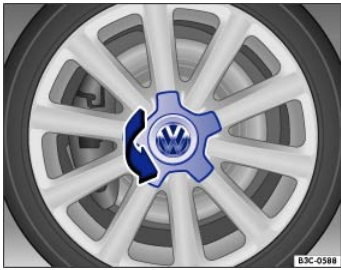
Fig. 188 Twisting the hubcap off.
