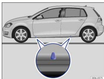
Fig. 193 Lift points for the jack.
