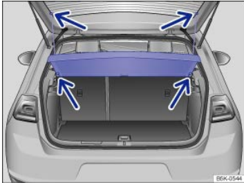
Fig. 147 In the luggage compartment: Installing and removing the luggage compartment cover.
