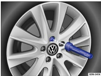
Fig. 197 Changing a wheel: Remove previously loosened wheel bolts using the screwdriver handle.
