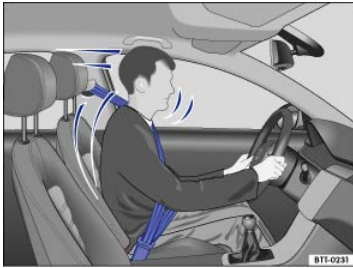
Fig. 30 Belted driver secured by the correctly worn safety belt in the event of a sudden braking maneuver.
