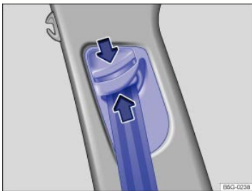
Fig. 35 Next to the front seats: Safety belt height adjuster.
