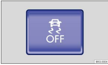
Fig. 130 In the lower center console: Button for switching ASR or ESC Sport mode on and off manually (if equipped).
