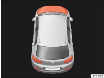
Fig. 174 In the instrument cluster display: Engine hood open or not properly closed.
