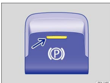
Fig. 119 In the lower center console: Electronic parking brake switch.
