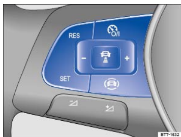
Fig. 113 Left-hand side of the multi-function steering wheel: Buttons for operating the Adaptive Cruise Control (ACC).
