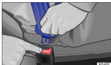
Fig. 32 Releasing the buckle tongue from the belt buckle.
