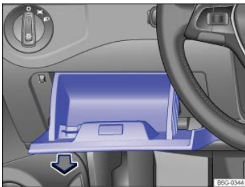
Fig. 162 On the driver side in the instrument panel: Removing the storage compartment to access fuses.
