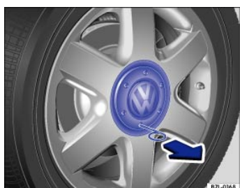
Fig. 187 Pulling the hubcap off.
