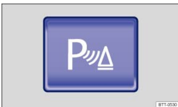
Fig. 121 In the lower center console: Button to switch the Park Distance Control system on or off.
