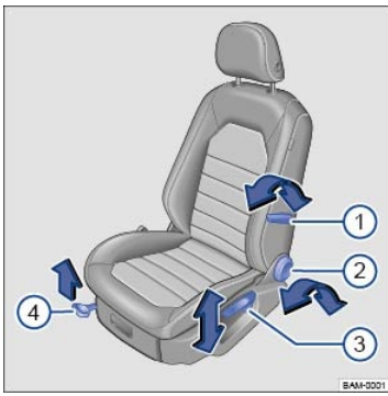
Fig. 71 Driver seat: Manual seat adjustment controls.
