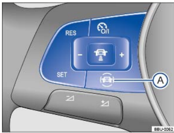
Fig. 20 On the multi-function steering wheel: Driver assistance systems button.
