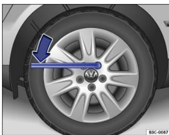
Fig. 191 Changing a wheel: Loosening the wheel bolts.
