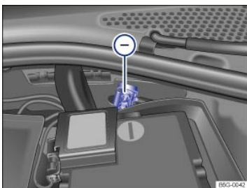
Fig. 166 In the engine compartment: Negative jump-start terminal ⊖.
