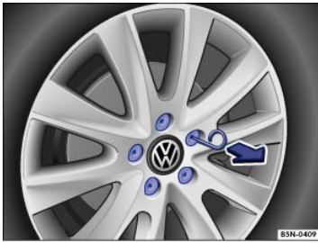
Fig. 190 Pulling cover caps off wheel bolts.
