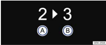
Fig. 95 In the instrument cluster display: Gear recommendation.
