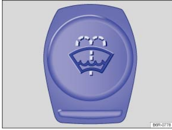
Fig. 175 In the engine compartment: Cap of the windshield washer fluid reservoir.
