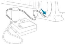
► Connect the hose from the bottle of sealant to the valve of the tyre to be repaired and tighten firmly.
