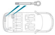
Depending on version, the towing eye is stored either in the interior trim of the boot sill, left-hand side, or in a bag behind the left-hand rear seat.
