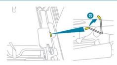
► Lift the vellow lever G. located on the righthand side, as far upwards as possible to unlock the seat
