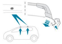
You must only attach the transverse bars to the four fixing points located on the roof frame.
