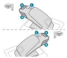
A. Button P To put the gearbox into Park mode.
