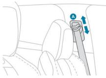
► To adjust the height of the anchorage point, squeeze control **A** and slide it to the notch desired.
