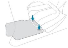
When fitting it on the driver's side, only use the mountings present on the carpet (a "click" indicates proper locking).
