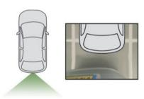
The camera records the vehicle's surroundings during the manoeuvre in order to create a view from above the rear of the vehicle in its near surroundings, allowing the vehicle to be manoeuvred around nearby obstacles.
