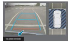
With the engine running and the speed below 12 mph (20 km/h), the system is activated via the **Driving/Vehicle** touch screen menu:
