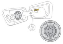
When a petrol filler nozzle is introduced into the fuel filler neck of a Diesel vehicle, it comes into contact with the flap. The system remains closed and prevents filling.
