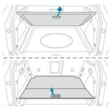
► Lift the boot floor as far as possible or lift the articulated boot mat (depending on version) to access the storage well.
