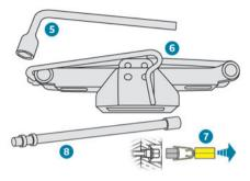
Wheelbrace For removing the wheel trim and the wheel bolts.
