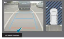
The system activates automatically when reverse gear is engaged.
