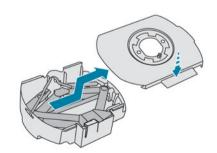
The tool box is installed at the centre of the spare wheel beneath the vehicle.
