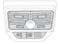
When this function is activated, the rear air vents blower starts up. In this case, the rear passengers can control the air flow from these air vents independently of the air conditioning air flow control for the front air vents.
