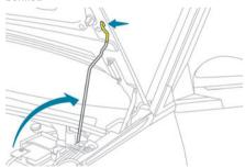
► Unclip the stay from its housing and place it in the support slot to hold the bonnet open.
