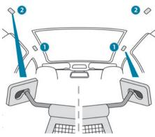
This removable net allows the entire loading volume up to the roof to be used:
