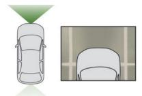
The camera records the vehicle's surroundings during the manoeuvre in order to create a view from above the front of the vehicle in its near surroundings, allowing the vehicle to be manoeuvred around obstacles nearby. This view is available with AUTO mode or in the
