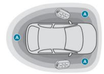
This system allows the unlocking, locking and starting of the vehicle, while carrying the electronic key on your person in the recognition zone A
