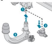
▶ Below the rear bumper, remove the protective plug 2 from the carrier 1.
