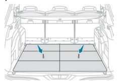
▶ Pull one of the straps; the 3 sections of the corresponding panel fold into concertina form. When the 3<sup>rd</sup> row seats are straightened, these folded concertina panels can be left upright or flat behind the seats (freeing up the seat well as a storage space).
