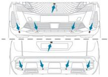
With the engine running, these systems allow views of your vehicle's close surroundings to be displayed on the touch screen using one camera for Visiopark 1 and two cameras for Visiopark 2.
