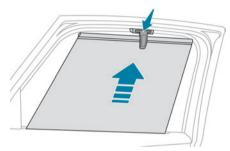
Fitted to the second row windows, they protect the passenger compartment from the sun's rays.
