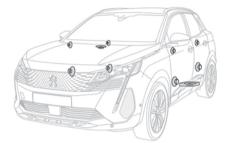
The vehicle is equipped with a high-fidelity acoustic system from the French brand FOCAL®. 10 speakers incorporating exclusive FOCAL® technologies offer the pleasure of pure and detailed sound inside the vehicle:
