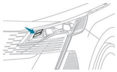
With the dipped or main beam headlamps on, this function allows headlamps to illuminate the inside of a bend using light-emitting diodes (LEDs).
