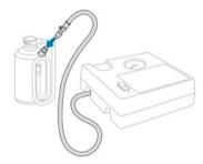
► Connect the pipe from the compressor to the bottle of sealant.
