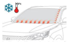
In cold weather, this system heats the bottom of the windscreen, as well as the area alongside the left-hand windscreen pillar.
