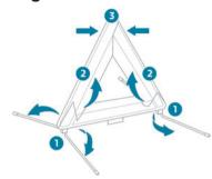
For versions supplied with a triangle as original equipment, refer to the illustration above. For other versions, refer to the assembly instructions provided with the triangle.
