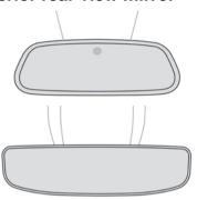
The electrochrome system uses a sensor that detects the level of exterior brightness and that coming from the rear of the vehicle, in order to automatically and gradually switch between day and night usage.
