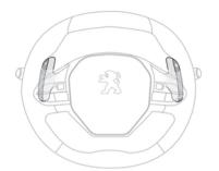
► Pull the "+" or "-" paddle towards you and release to shift up or down a gear, respectively.
