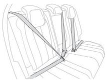
Each of the rear seats has a three-point seat belt with inertia reel.
