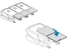
Each seat has a continuity panel at the bottom of the backrest, which, once unfolded:
