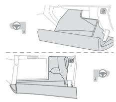
It houses the front passenger airbag deactivation switch.
