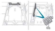
When there is a seat at the back of the boot, the removable support is fixed against the front wall of its housing.
