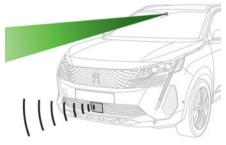
The vehicle has a camera located at the top of the windscreen and, depending on version, a radar located in the front bumper.
