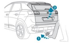
► Position yourself behind the vehicle by the number plate and perform a "kicking" movement in the "**OK**" detection zone.
