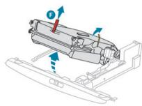
▶ While keeping the yellow lever held up as far as possible, raise the rear part of the seat using the red strap F.
