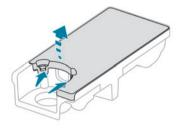
▶ Unclip the two fixings to open its cover.
