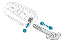
► To eject the key or put it back in place, pull and hold the button
