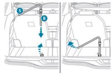
► Fold up the concertina panel and install the third row seat, on the left-hand side (if the vehicle is equipped with it).
