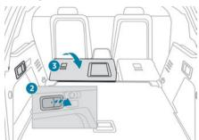
► Pull the backrest release lever 2 towards you. The backrest 3 folds fully onto the cushion.
