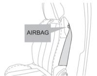
In the event of a serious side impact, this system protects the driver and front passenger to mitigate the risk of injury to the chest, between the hip and the shoulder.
