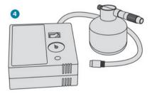
4. 12 V compressor with cartridge of sealant and speed limit sticker For temporary repair of a tyre and to adjust the tyre pressure.
