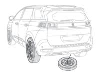
The spare wheel is held by a winch system underneath the rear of the vehicle.
