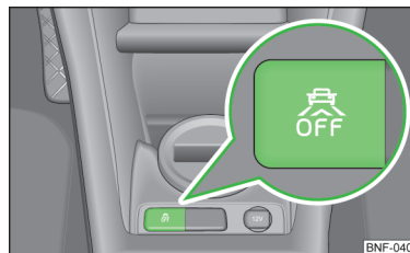
Fig. 90 Lower part of the centre console: Button for the City Safe Drive system
