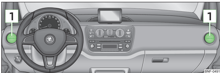
Fig. 73 Air outlet vents
