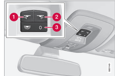
Light switches, front roof lighting
