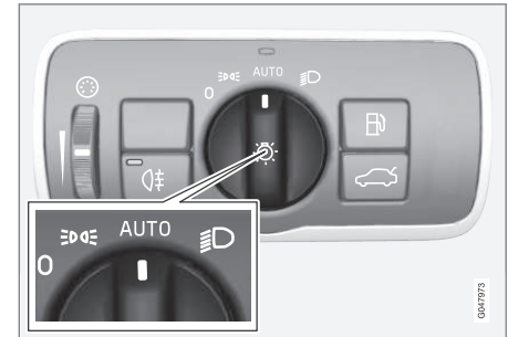
Headlight switch in the AUTO position
