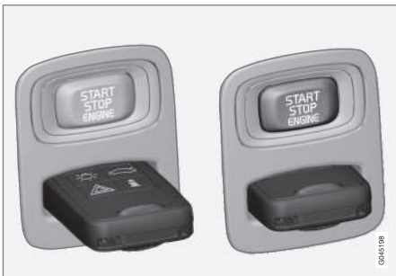
Ignition switch with remote control key extracted/inserted.
