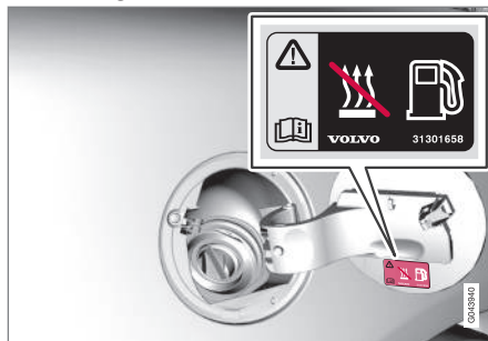
Warning label on fuel filler flap.
