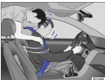
Fig. 57 Unbelted passengers in the rear seats are thrown forward on top of the belted driver.
