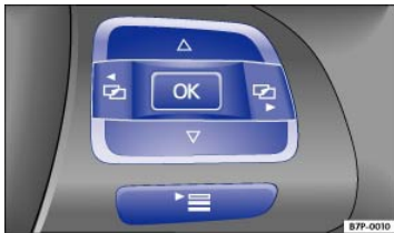
Fig. 13 Right side of the multi-function steering wheel: Controls for the menus in the instrument cluster.
