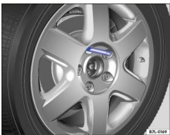
Fig. 215 Changing a wheel: Mounting pin in wheel bolt hole closest to the top.
