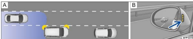
Fig. 157 Driving with Side Assist: A: Moving to another lane with rear traffic. B: Side Assist indicator lights in the left outside mirror.
