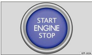
Fig. 131 In the front center console: Starter button of the Keyless Access locking and starting system.
