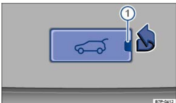
Fig. 202 Inside the luggage compartment: Remove the cover plate in the trunk lid.
