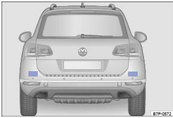
Fig. 156 Rear view of the vehicle: Areas of the Side Assist radar sensors.
