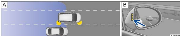
Fig. 158 Driving with Side Assist: A: Passing another vehicle and moving to the right lane. B: Side Assist indicator lights in the right outside mirror.
