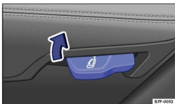
Fig. 96 Lower part of the rear seat bench: Lever to unlock the rear seat backrest by hand.
