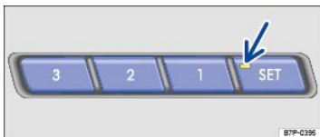
Fig. 51 Memory buttons in the upper part of the driver and front passenger doors.
