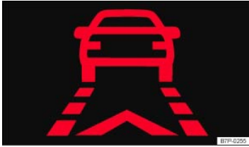
Fig. 151 In the instrument cluster display. Warning: Distance to vehicle ahead becoming too small.
