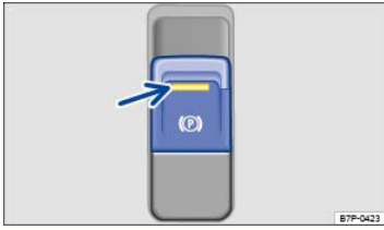
Fig. 136 In the lower front center console: Switch for the electronic parking brake.
