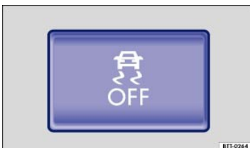
Fig. 137 In the front center console: Button to manually switch ASR on and off.
