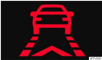
Fig. 149 In the instrument cluster display. Advance warning: Distance to vehicle ahead becoming too small.
