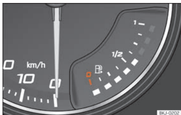
Fig. 65 Analogue instrument panel: fuel gauge
