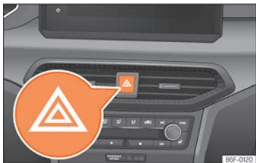
Fig. 95 Dash panel: hazard warning lights switch
