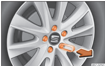
Fig. 33 Wheel: wheel nuts with caps.
