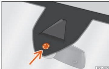
Fig. 100 Rain sensor sensitive surface
