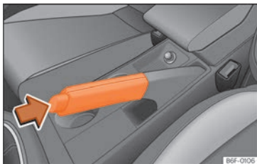
Fig. 162 Handbrake between the front seats.
