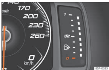
Fig. 66 Digital instrument panel: fuel gauge.
