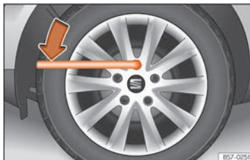
Fig. 35 Wheel change: loosen the wheel nuts.
