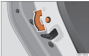
Fig. 88 Childproof lock on the left hand side door.
