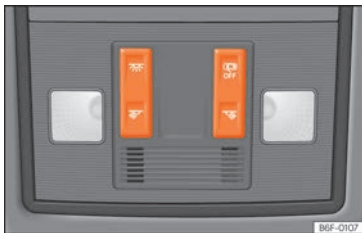
Fig. 97 Detail of roof lining: front lighting of the passenger compartment.
