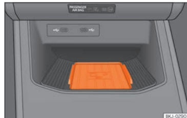
Fig. 127 In the centre console: pad for the mobile phone connection.
