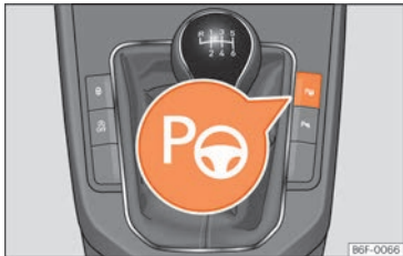
Fig. 163 In the centre console: button to switch on the Park Assist system.
