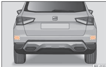
Fig. 142 Rear view of the vehicle: radar sensor zones.
