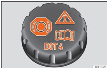
Fig. 199 Engine compartment: brake fluid reservoir cap.
