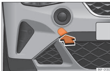
Fig. 44 Right side of the front bumper: remove the cover.
