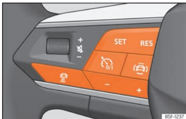
Fig. 149 On the multifunction steering wheel: buttons to operate the ACC
