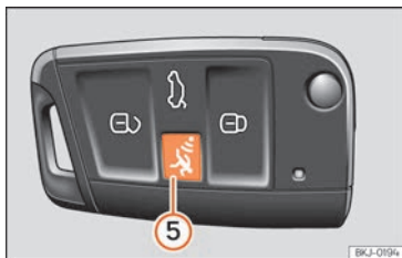
Fig. 78 Vehicle key with alarm button.
