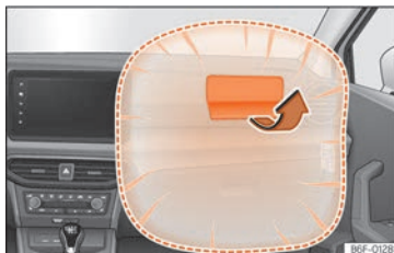
Fig. 15 Front passenger airbag located in dash panel.
