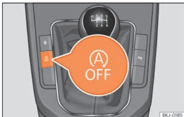
Fig. 132 Centre console: Start-stop system button.
