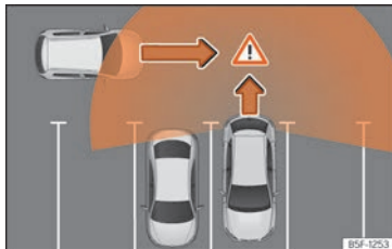
Fig. 161 Schematic representation of the rear cross traffic alert assistant: zone monitored around the vehicle while leaving a parking space.
