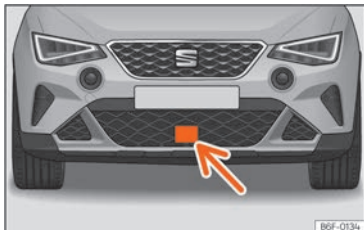
Fig. 139 On the front bumper: radar sensors.
