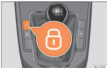
Fig. 82 Centre console: central locking button.
