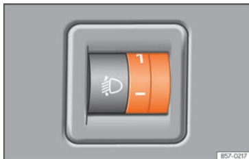
Fig. 96 Next to the steering wheel: headlight range control.
