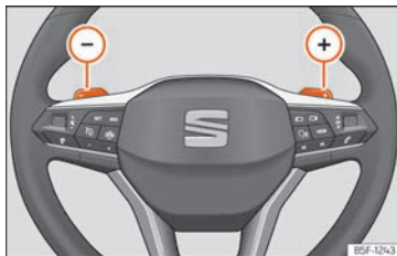
Fig. 136 Steering wheel: automatic transmission levers
