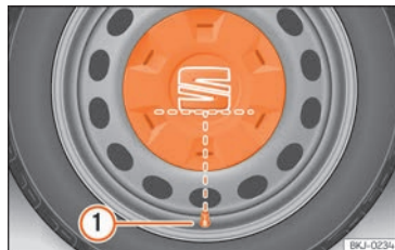
Fig. 32 Correct positioning of the central wheel trim for steel rims.
