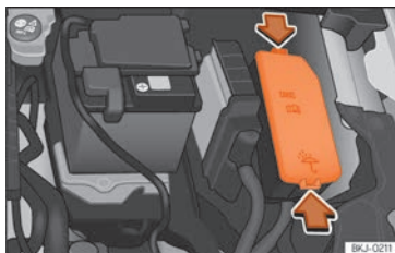
Fig. 49 In the engine compartment: fuse box cover.
