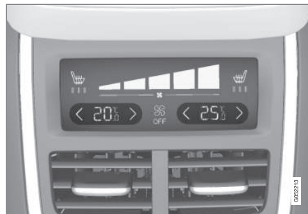
Temperature controls on the climate panel on the rear side of the tunnel console
