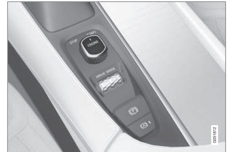
Start knob in the tunnel console
