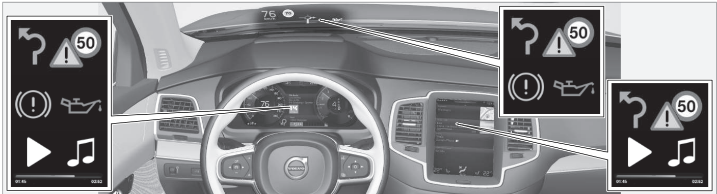
Information is presented in different displays depending on how it should be prioritized
