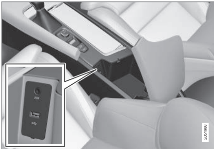
USB socket in the tunnel console
