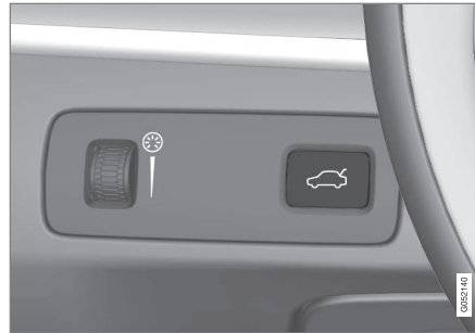
Button on the lighting panel in the passenger compartment
