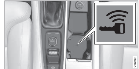
Back-up reader in the tunnel console
