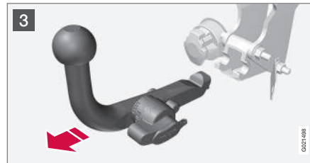
3 Turn the locking wheel down fully, until it comes to a stop. Hold it in this position while pulling the towbar rearward and upward.
