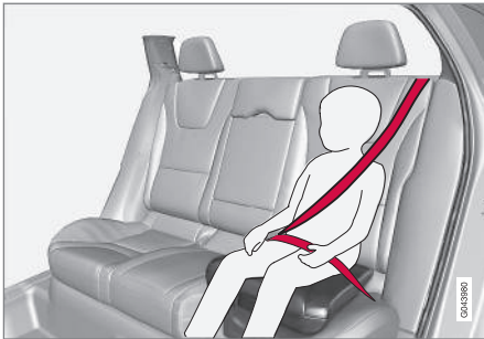
Correct position, the seatbelt should be positioned on the shoulder.
