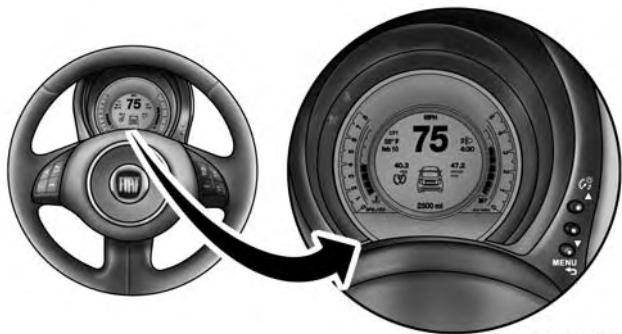
Electronic Vehicle Information Center (EVIC) Display
