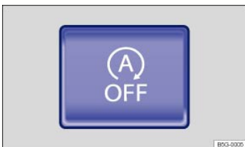
Fig. 109 In the lower center console: Button for the Start-stop system.
