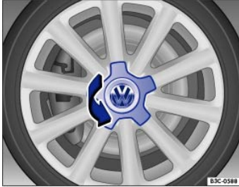
Fig. 192 Twisting the hubcap off.
