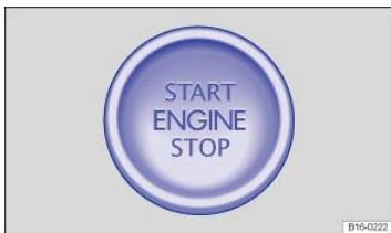
Fig. 106 In the lower center console: Starter button for the Keyless Access system.
