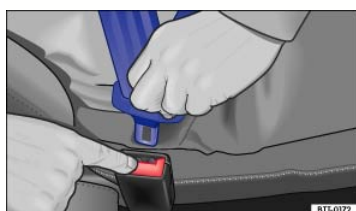
Fig. 30 Releasing the buckle tongue from the belt buckle.
