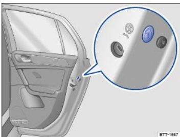
Fig. 67 On the front side of the rear passenger door: Manual lock, covered by a rubber seal.
