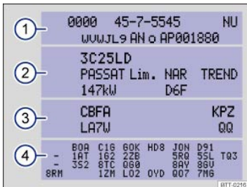
Fig. 203 Vehicle identification label: Shown in the example with engine identification code CBFA ③.
