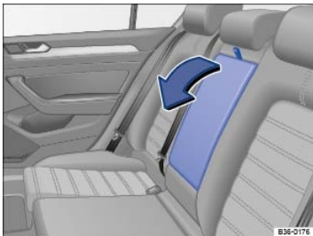
Fig. 89 Folding down the rear center armrest (arrow).
