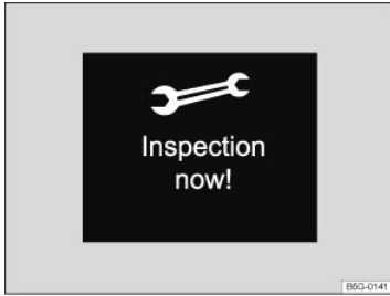
Fig. 15 In the instrument cluster display: Example of the service reminder when a service is due.
