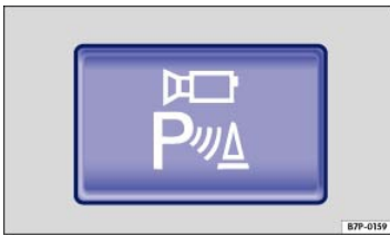
Fig. 125 In the upper center console: Button to switch the Park Distance Control system on or off (vehicles with Area View).
