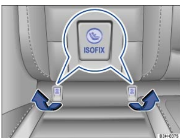
Fig. 49 On the rear outboard seat backrests: Removing the covers (if equipped) on the LATCH/UCRA lower universal anchorages.
