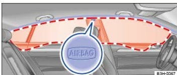
Fig. 41 On the left vehicle side: Installation location and deployment zone of the Side Curtain Protection airbag.
