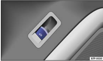
Fig. 64 In the driver door: Switch for opening the trunk lid.
