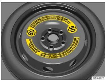
Fig. 189 In the luggage compartment: Compact spare wheel (label design may vary).
