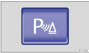
Fig. 124 In the upper center console: Button to switch the Park Distance Control system on or off (vehicles without Area View).
