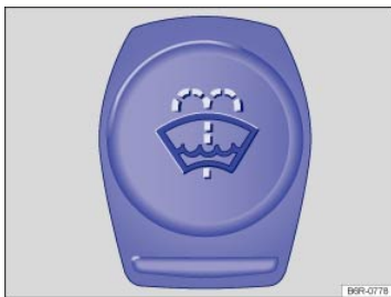
Fig. 177 In the engine compartment: Cap of the windshield washer fluid reservoir.
