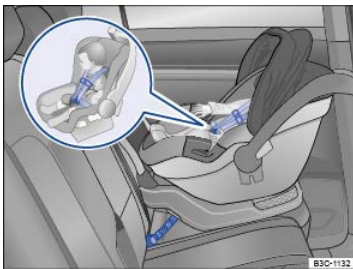
Fig. 46 Example of a rearward-facing infant seat properly installed on the rear seat.
