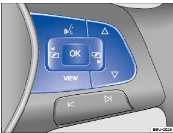
Fig. 17 Right side of the multi-function steering wheel: Controls for the menus and information in the instrument cluster display.
