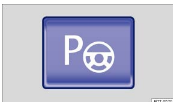
Fig. 130 In the lower center console: Button for switching on the Park Assist system.
