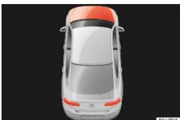
Fig. 176 In the instrument cluster display: Engine hood open or not properly closed.
