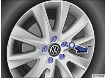
Fig. 194 Pulling cover caps off wheel bolts.
