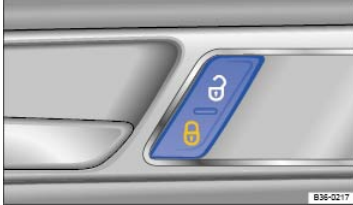
Fig. 63 In the driver and passenger doors: Power locking switch.
