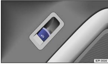
Fig. 71 In the driver door: Switch to open the trunk lid.
