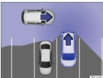
Fig. 134 Rear Traffic Alert: Monitored area around the vehicle that is backing out of a parking space.
