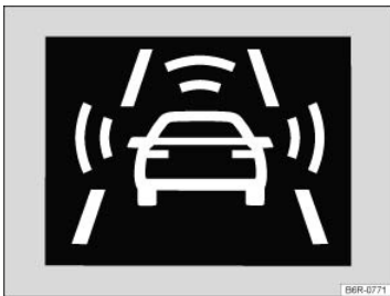
Fig. 120 In the instrument cluster display: Advance warning (symbol displayed in color on an instrument cluster with color display).
