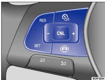
Fig. 115 Left-hand side of the multi-function steering wheel: Buttons for operating the cruise control.
