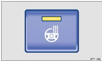
Fig. 100 In the lower center console: Button for steering wheel heating.
