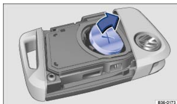
Fig. 57 Remote control vehicle key: Opening the battery compartment cover.
