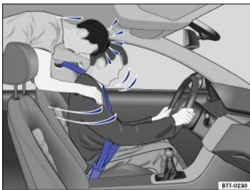
Fig. 27 Unbelted passengers in the rear seats are thrown forward on top of the belted driver.
