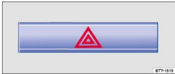
Fig. 53 In the center of the instrument panel: Button for the emergency flashers.
