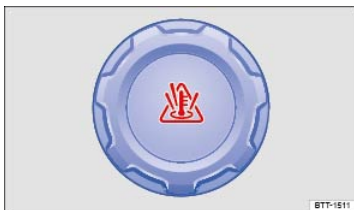
Fig. 181 Coolant expansion tank cap in the engine compartment.
