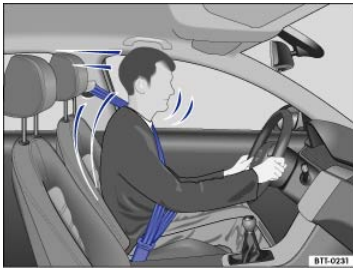
Fig. 28 Belted driver secured by the correctly worn safety belt in the event of a sudden braking maneuver.
