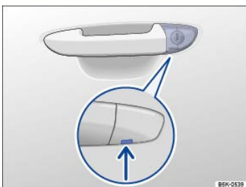
Fig. 65 Driver door: Concealed lock cylinder.
