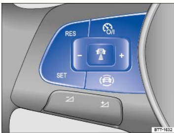
Fig. 118 Left-hand side of the multi-function steering wheel: Buttons for operating the Adaptive Cruise Control (ACC).
