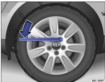
Fig. 195 Changing a wheel: Loosening the wheel bolts.
