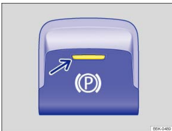
Fig. 123 In the lower center console: Electronic parking brake switch.
