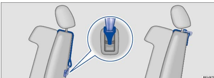
Fig. 51 Example of a mounted upper tether strap: The version on the left shows an outer seating position. The version on the right shows the center seating position.
