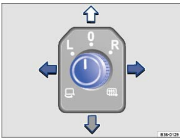
Fig. 97 In the driver door: Adjusting knob for the outside mirrors.
