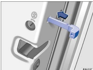
Fig. 68 On the front side of the rear passenger door: Locking the vehicle with the emergency key.
