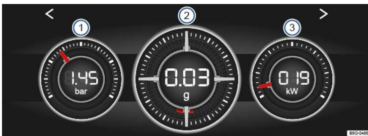
Fig. 19 In the Infotainment system: Performance Monitor sport gauges (if equipped). Gauges shown in the display may vary depending on configuration.
