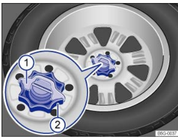
Fig. 188 In the luggage compartment: Handwheel holding the spare wheel in place (if equipped).
