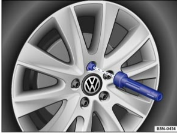
Fig. 200 Changing a wheel: Remove previously loosened wheel bolts using the screwdriver handle.
