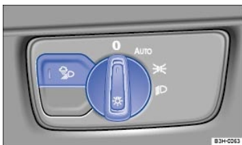
Fig. 91 Headlight switch next to the steering wheel (with poor weather lights and automatic headlights, if equipped).
